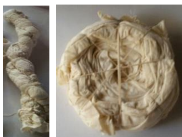
Fig. 1: Tied for Copper Sulphate mordanting
